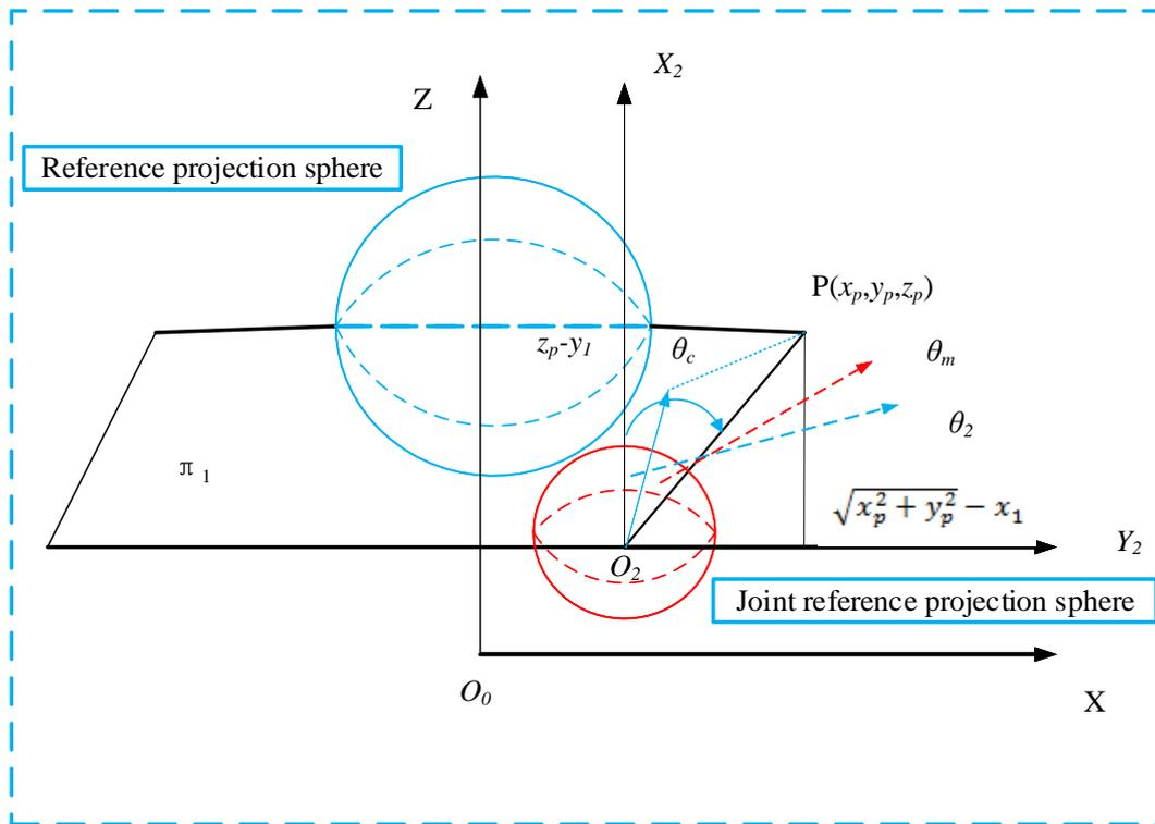
Figure 3: Sketch map of solving the first solution of the second joint angle
