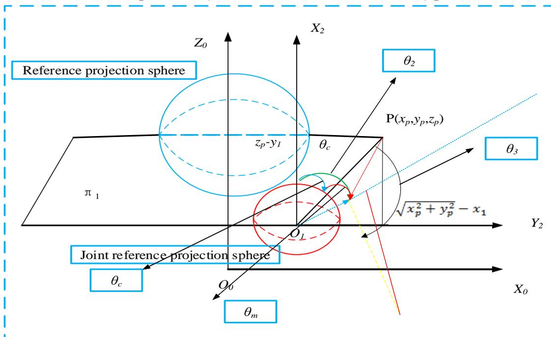
Figure 4: Sketch map of solving the second solution of the second joint angle
