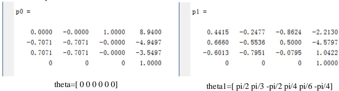
**Figure 7:** Pose matrix of robot body generated after program operation
