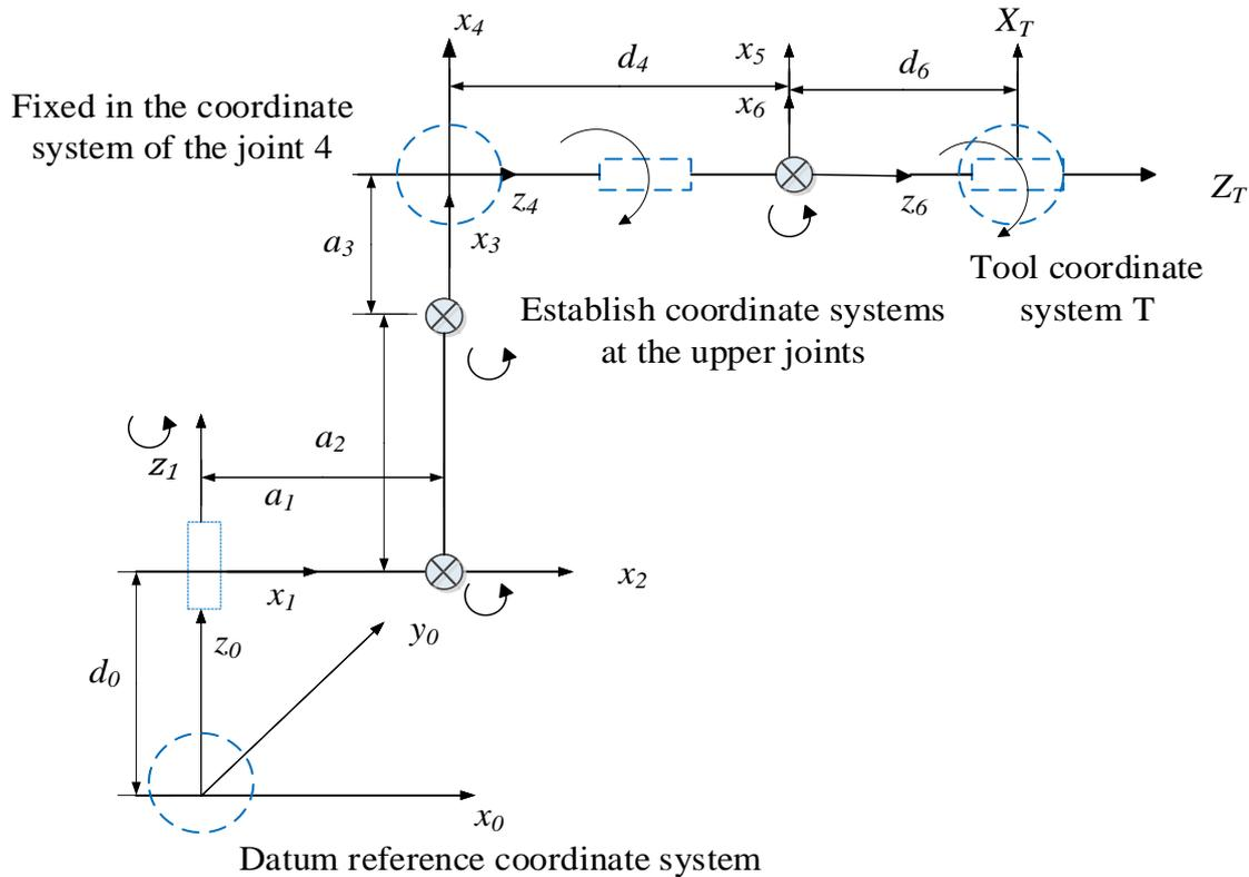
Figure 1: Sketch map of robot body kinematics coordinate system
