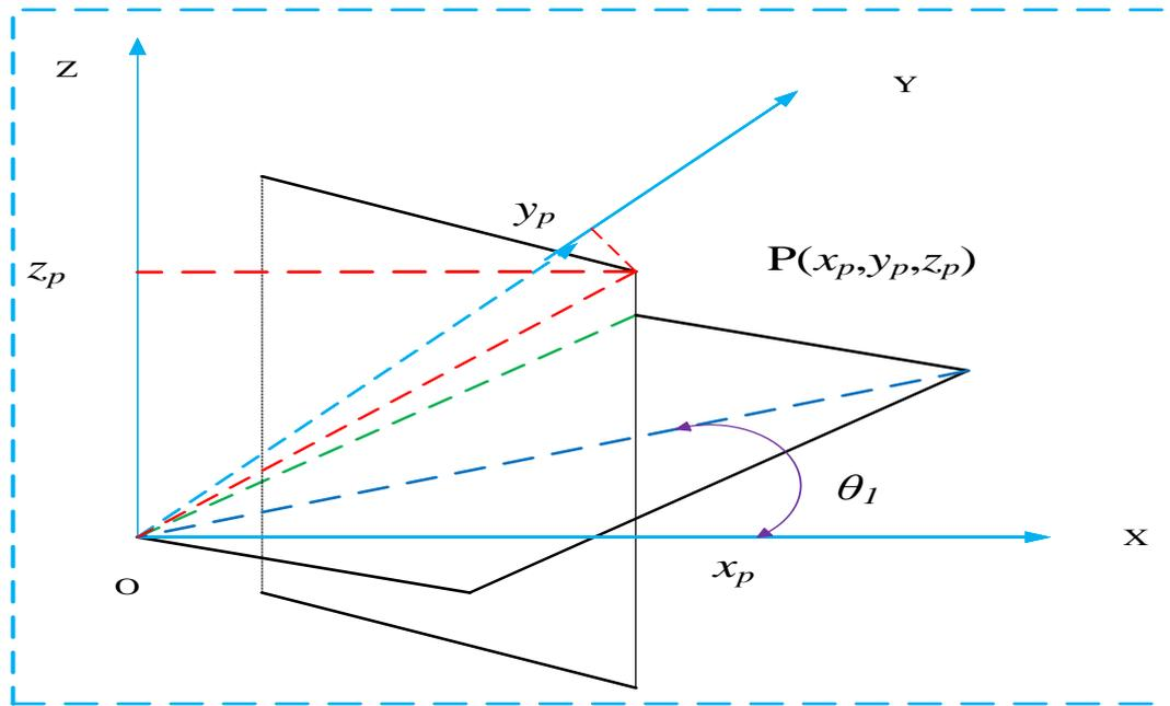
Figure 2: Sketch map of solving the first joint angle
